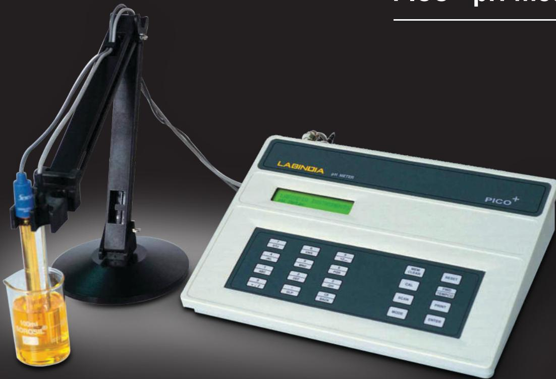
This bench-top pH meter is an ideal help in every laboratory for routine or R&D level measurement. This very handy instrument measures pH, mV and has 40- point data memory storage.
